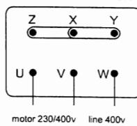
**Y/Δ STARTING.** Remove the bridge plates from the terminal box and connect the motor terminals to the corresponding ones on the starter.
