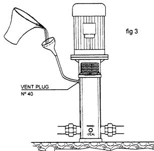
After connecting and filling, start the pump with the delivery gate valve closed and check that the rotation direction is correct (shown on the adapter and coupling) through the coupling protection or fan cover.
