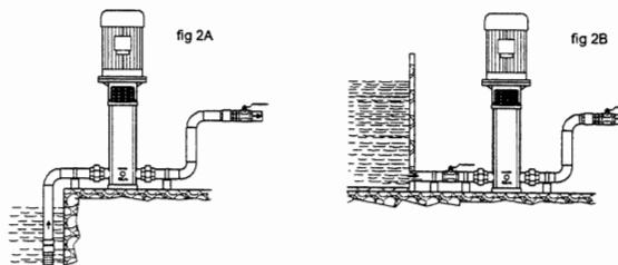
**WARNING:** Provide space around the pump for motor ventilation, to allow for checking of shaft rotation, for filling and draining the pump and to allow for collection of the liquid to be removed
